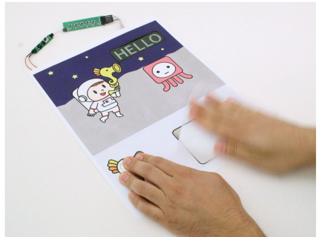
Figure 1. Paper Generator harvests energy from rubbing and activates the e-paper display, revealing the word “hello”.
