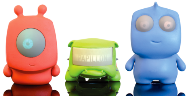
Figure 1. Curved displays are embedded into the characters to design interactive eyes. The characters are passive and do not have any electronics embedded.
