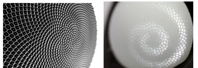
Figure 5. spheric display surfaces with Fibonacci pixel arrangements.
